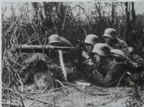
Figure 13: A Maxim machine gun, belt-fed and water-cooled, operated by German infantrymen, World War I.
